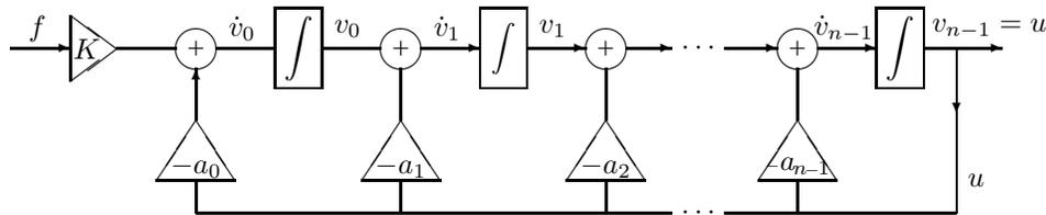
The diagram is the result of the fact, that the filter is represented by the linear differential equation
